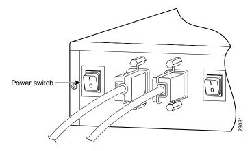
The Cisco RPS provides power in 10 to 15 seconds. The Cisco RPS is working properly when all its front-panel LEDs are solid green. If the external device does not power up, refer to troubleshooting section of the *Cisco Redundant Power System Hardware Installation Guide* on Cisco.com.
